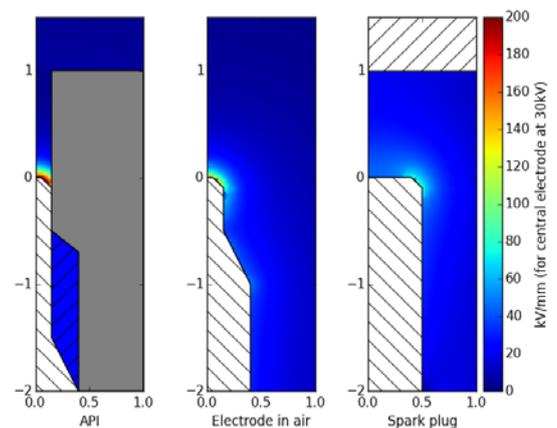
Figure 6: Electrostatic simulation showing the effect of a dielectric material (gray area) on the electric field of a wire at 30 kV. Cylindrical symmetry is assumed.
