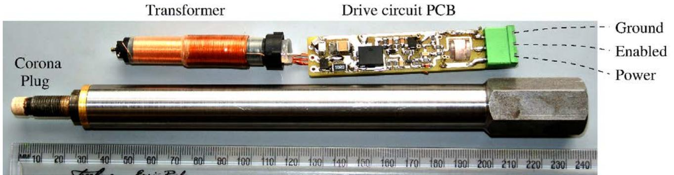
Figure 5: Photo of first API laboratory prototype.
