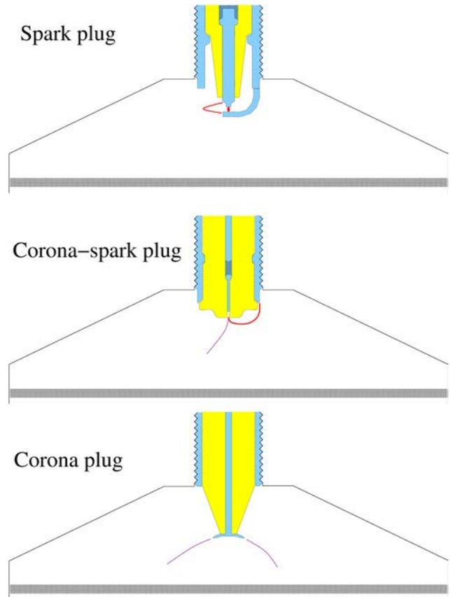
Figure 3: Cross-section of spark and corona plugs inside the combustion chamber
