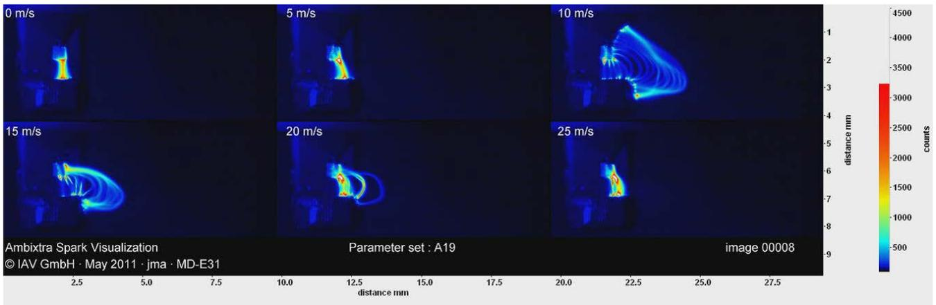
Figure 9: VSI spark visualisation at 1 bar pressure for different gas flow velocities.
