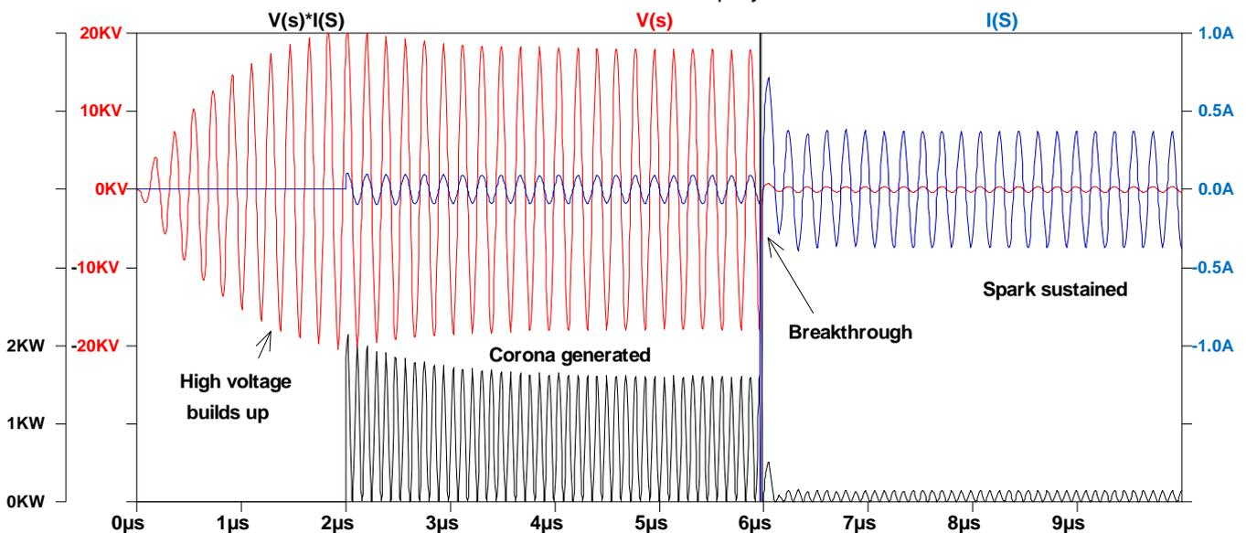
Figure 4: Voltage (red), current (blue) and power (black) waveforms during the three operating modes of API: High voltage build-up mode (left), corona generation mode (middle) and spark sustaining mode (right).
