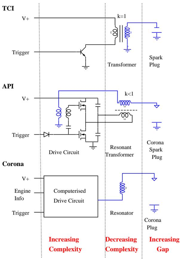
Figure 2: Circuit diagram of TCI, API and Corona Ignition
